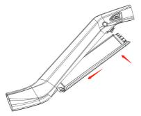
Push the top part of the battery into the frame, until you hear the battery lock into position, and turn the limiting stopper to keep the battery from dropping.
